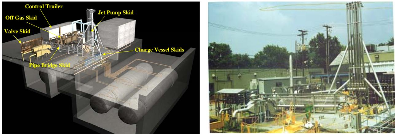
**Fig. 3. BVEST tank system CAD drawing layout and final system**
