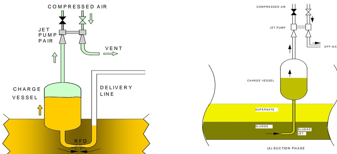
**Fig. 1. A simplified fluidic pumping and mixing arrangement**
