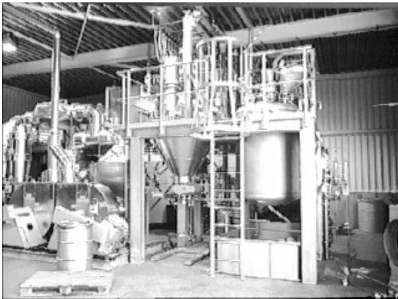
Pebble bed pyrolysis unit, as installed for cold testing at Belgoprocess
