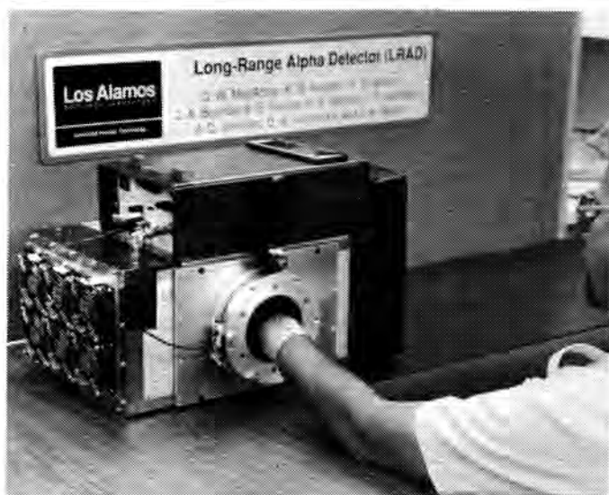
Fig. 6. Prototype of LRAD hand monitor.
