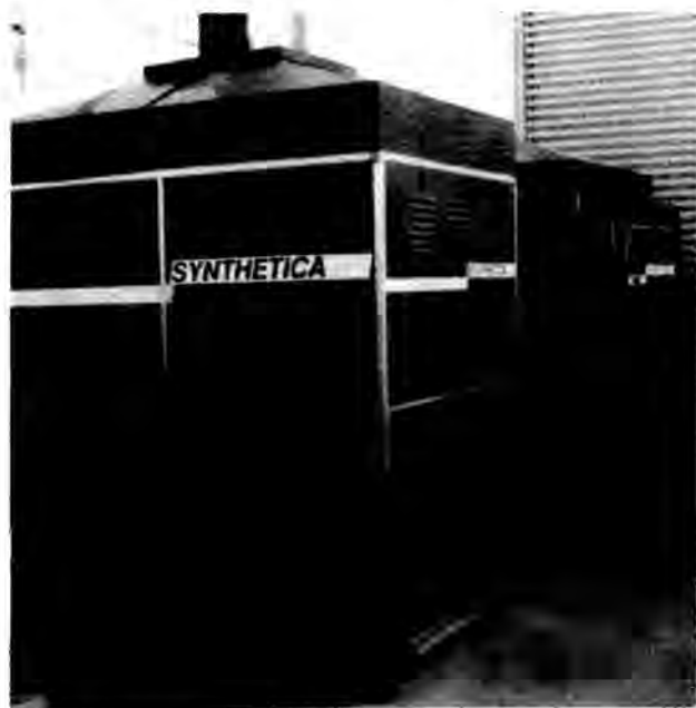
Fig. 4. Synthetica detoxifier coupled to drum feed evaporator.
