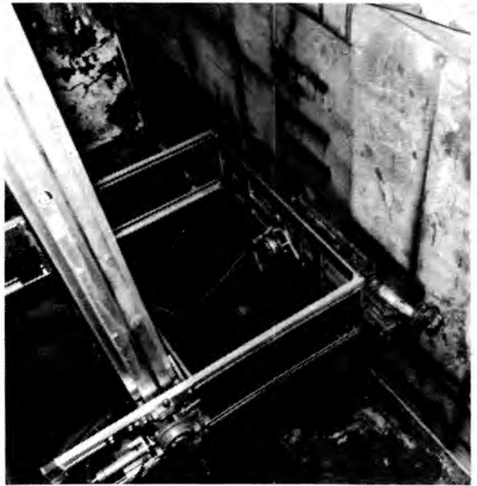
Fig. 8. Wall liner cutting torch in test cell.
