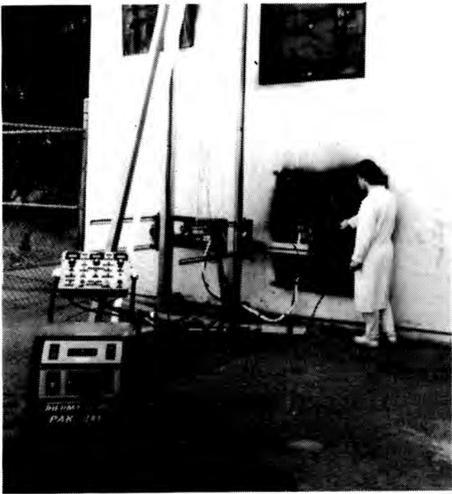
Fig. 7. Wall liner cutting torch mock-up test.
