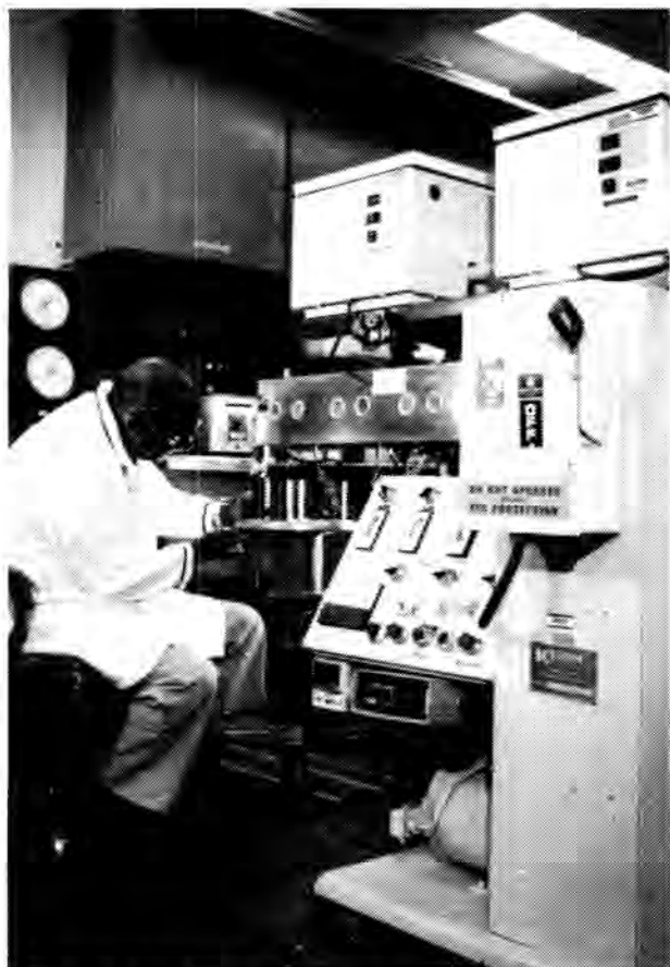
Fig. 1. BNL bench-scale extruder used to produce nitrate salt waste forms for testing.
