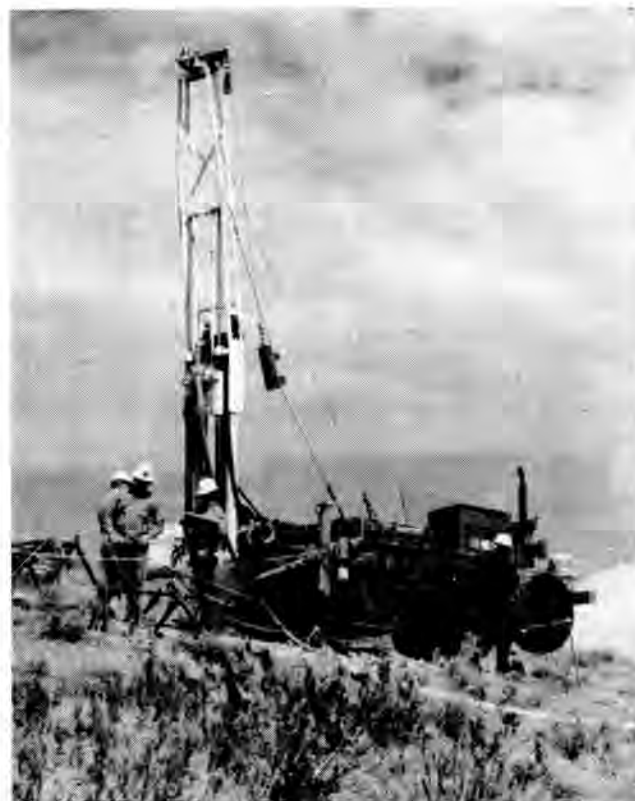
Fig. 1. A set of 12 shallow neutron access boreholes was completed in 1992 to evaluate natural infiltration by rainfall.
