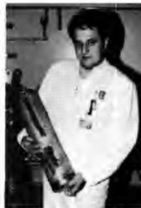
Fig. 4. Cesium selective ion exchange material is used in stainless steel columns with volume of 8 liters.
