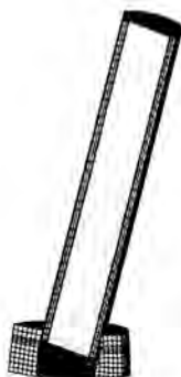
Fig. 6. Deformed truck cask after 9 m corner drop.
