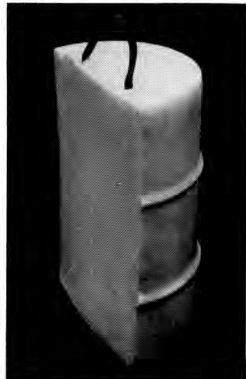
Fig. 6. Photograph of the polyethylene/sodium nitrate waste form produced during the production-scale feasibility test, showing the outer surface and cross-sectional view.
