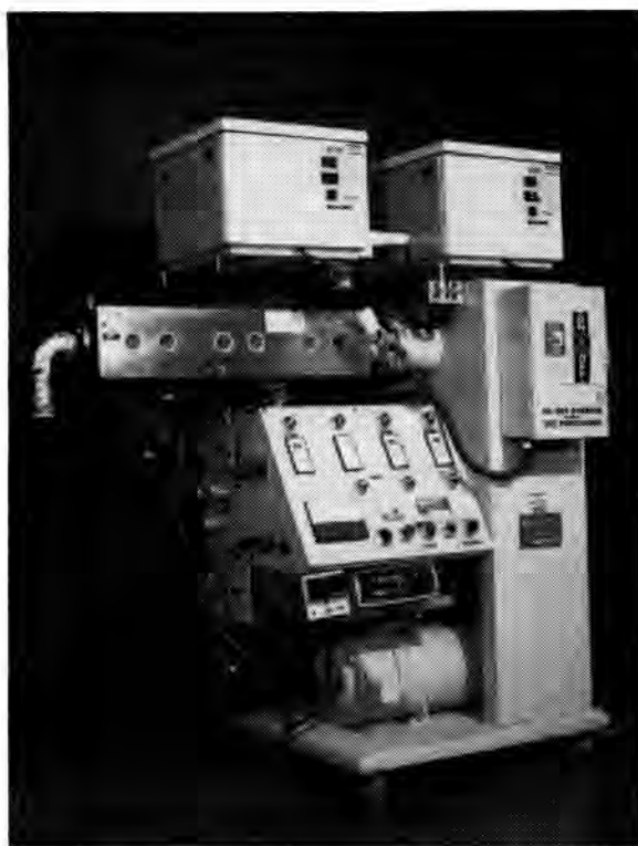
Fig. 2. Photograph of laboratory-scale extruder with separate dynamic feeders for waste and binder.
