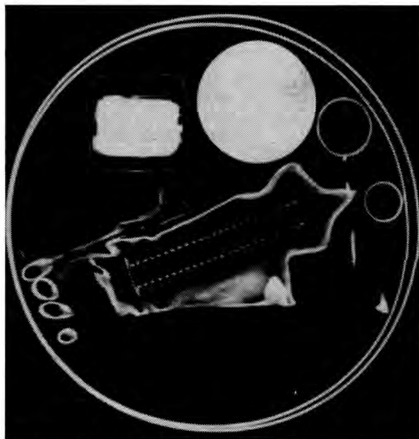
Fig. 9. The white circle in this 2 MeV CT image is the dense object at the bottom of the DR image. A lead-lined glove containing a filter is in the center.
