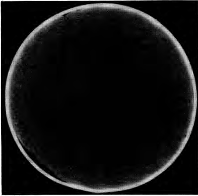
Fig. 20. This CT image shows a 60 cm diameter glass form. There are gaps between the glass and the container, and cracks in the glass.
