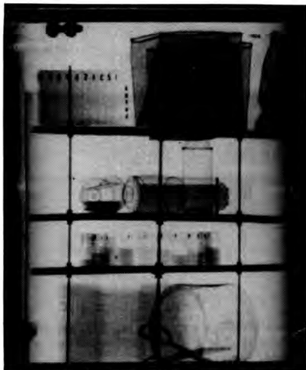
Fig. 10. This 420 kV DR image shows four layers, with separators supported by threaded rods between them. Many items are easily identifiable.
