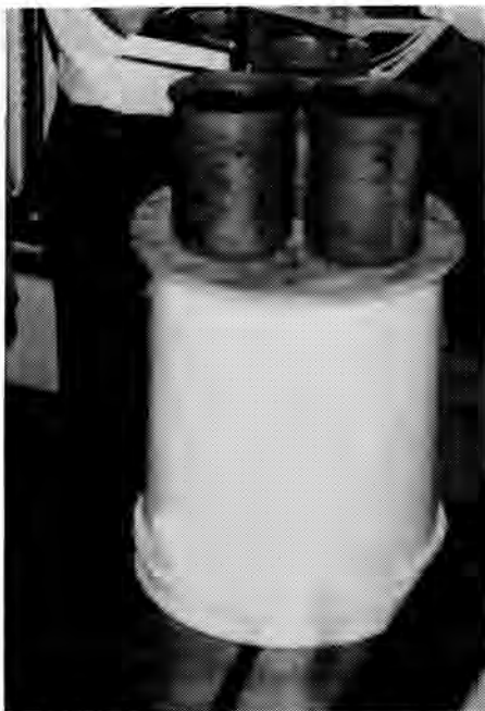
Fig. 15. This photo shows three stainless steel beakers mounted on the ACTIS turntable for scanning. The beakers contain a type of glass used to solidify high level radioactive waste.
