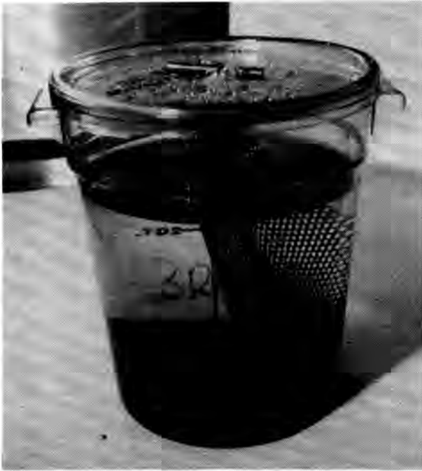
Fig. 1. Brunswick-1 mixed-bed resin waste-form specimen after being leached for 90 days, showing the typical geometry of decomposition waste form.
