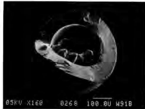
Fig. 4. SEM micrograph of Split Lewatit DN resin bead removed from 15 wt% Lewatit DN in OPC w/c = 0.45 sample.
