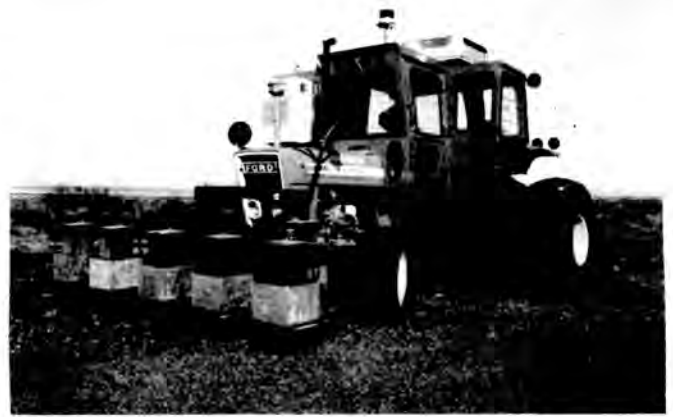
Fig. 4. A large area surface radioactive contamination monitor. This vehicle has five sensors mounted in the front to detect and map any radioactive contamination that may be present in the soil. This information is needed to determine what remediation activities should be conducted.
