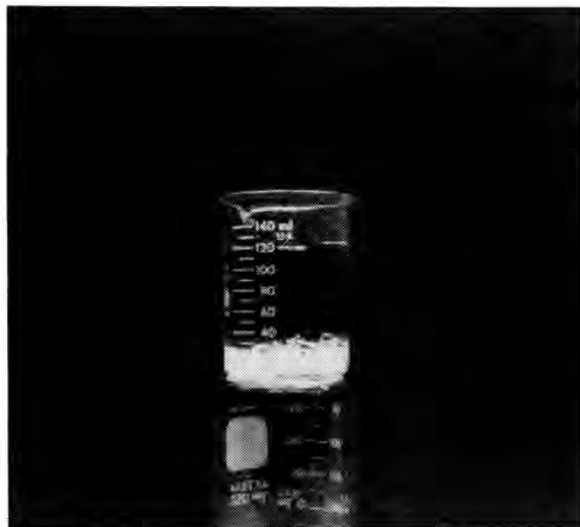
Fig. 2. Flotation of Polymethylmethacrylate (PMMA) Beads by Sparging with Nitrogen Gas: PMMA beads [density = 1.2 \text{ g}(\text{cm}^{-3}) ] in DI water before sparging with gas.
