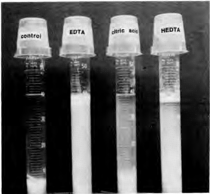
Fig. 5. Synthetic waste formulations 30 minutes after sparging with nitrogen gas.
