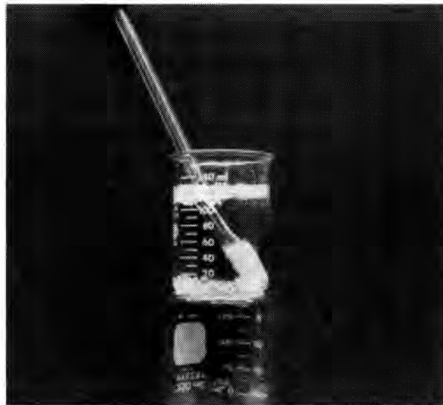
Fig. 3. The Flotation of PMMA beads by attachment of gas bubbles from a nitrogen sparge. The PMMA beads form a stable raft indefinitely after the cessation of the gas sparge.
