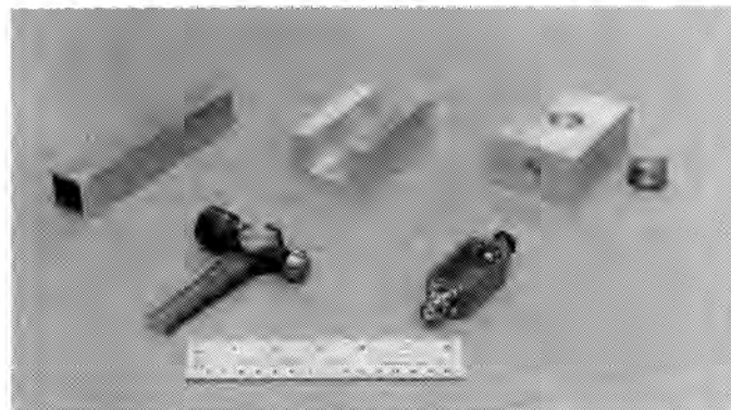
Fig. 13. Photograph of five typical solid waste configurations. Starting in the upper left corner and moving clockwise, they are a piece of pipe, an aluminum channel, an aluminum "pig" with a 1/2-in. hole drilled through it, a small Pomona® box, and a hammer head.
