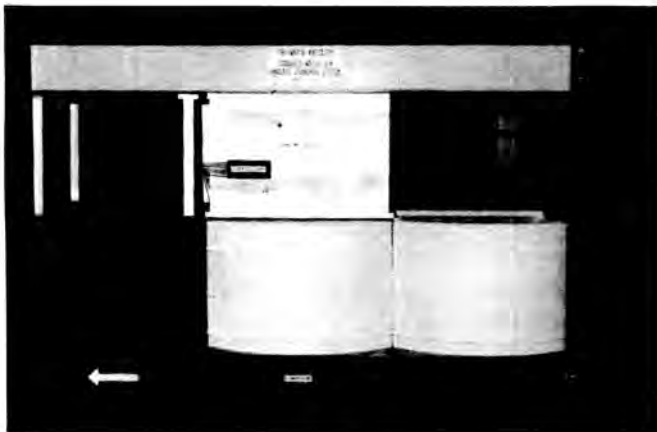
Fig. 2. SWB ready to receive TRU waste.
