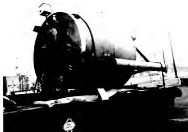
Fig. 2. Burial Tank (11,355 L) Requiring Fill Material.
