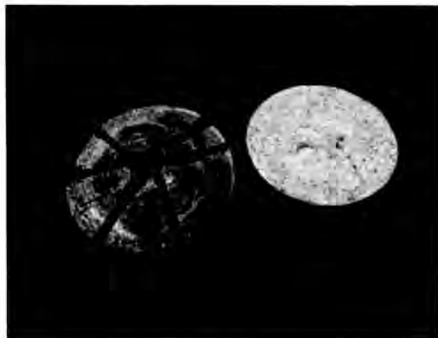
Fig. 6. Impact-Strength Test Specimens--Cement (left) versus Light-Weight, Reinforced Vermiculite-Concrete (right) Used for Solidifying Sodium Sulfate Liquid.
