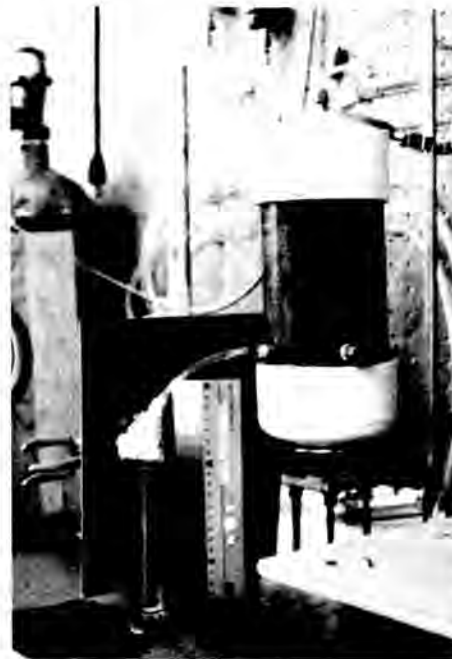
Fig. 5 Failure of a sample due to piping when outflow is permitted only through a side hole of 2.25 mm diameter.
