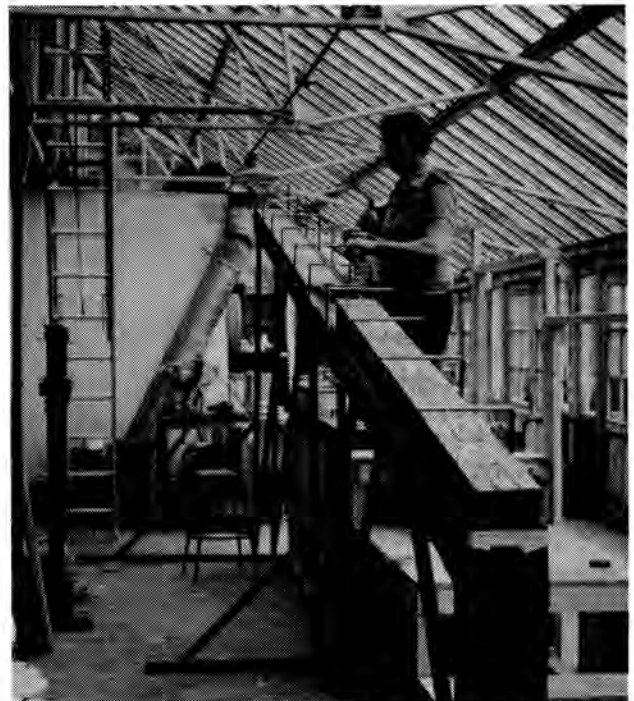
Fig. 18. Large Soil Beam Used for Final Selection of Diatomaceous Earth as Conductive Layer Material.
