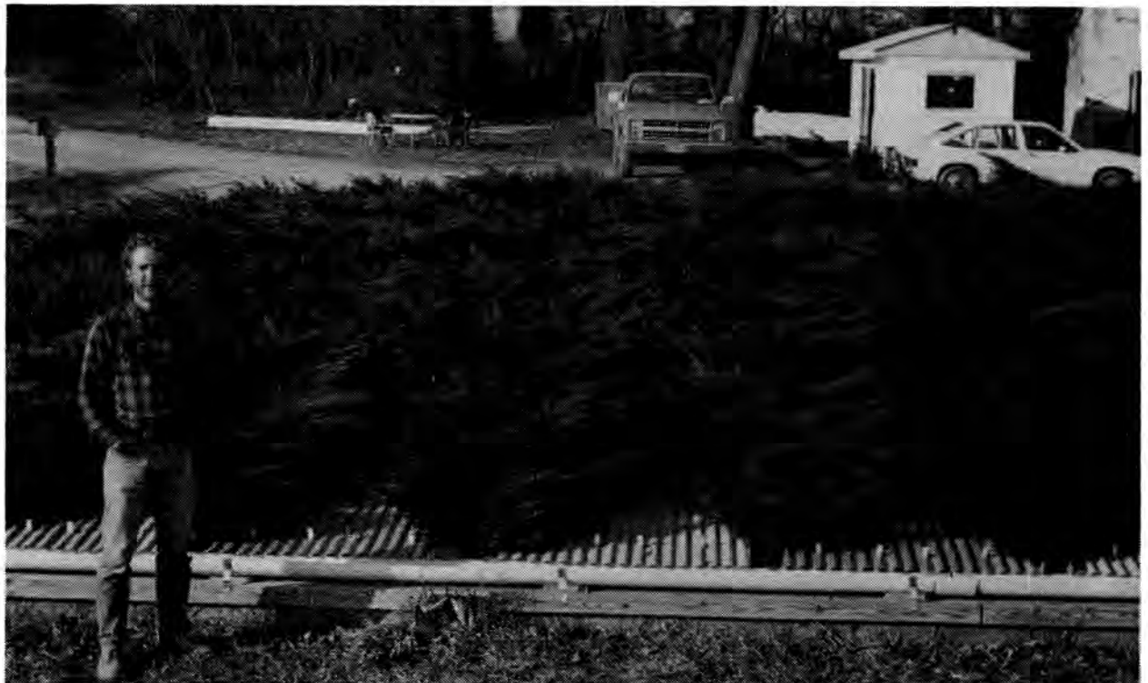
Fig. 5. Bioengineering Plots at Beltsville. Photo Taken in January of 1990, Three Years After Planting of Pfitzer Junipers. Run-off is 74% of Precipitation.
