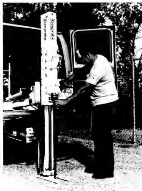
Fig. 4. Hydraulically-Powered Soil-Gas Sampling System Mounted in the Rear of a Cargo Van.
