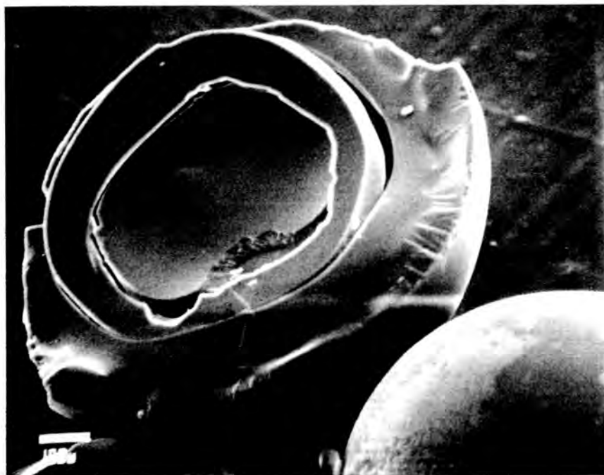
Fig. 1. SEM Photomicrograph of an EPICOR-II Strong Acid Cation Resin Bead From Strong Acid Cation Resin Bead From PF-8#1 at 100 Magnification.
