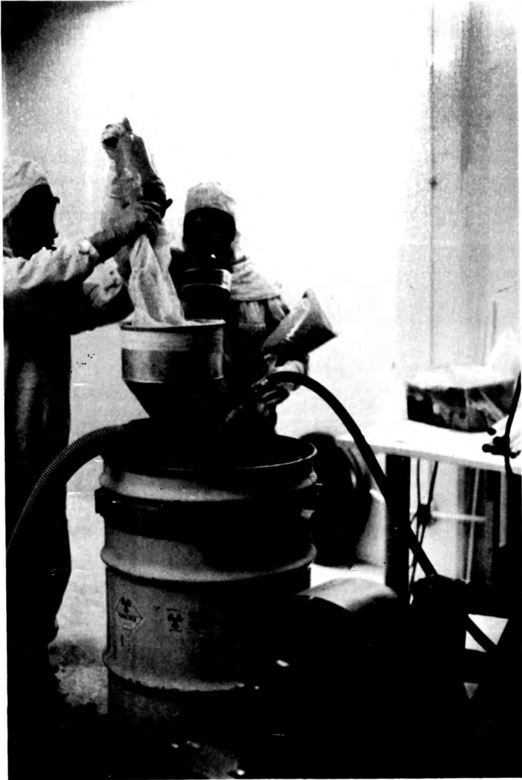
Fig. 1. An INEL Process has been Developed to Solidify and Stabilize Certain Mixed Wastes, such as the Incinerator Flyash Being Treated Here.
