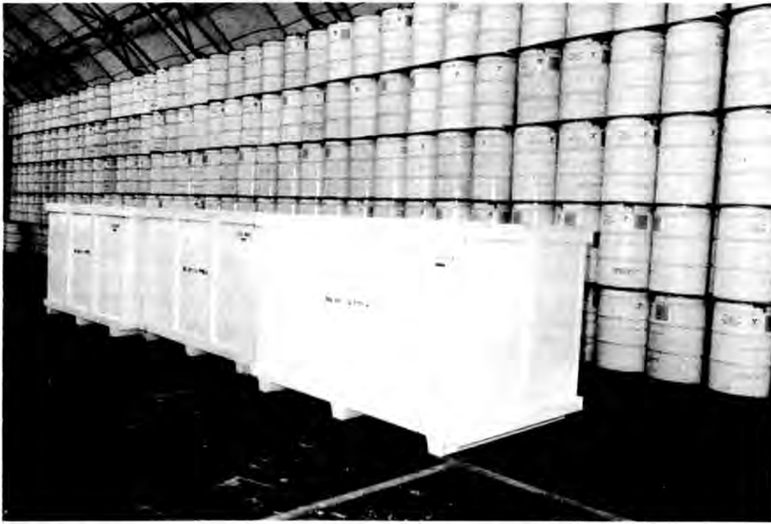
Fig. 2. The INEL Stores Many Thousands of Containers of Mixed TRU Waste in a Close-Packed Configuration.
