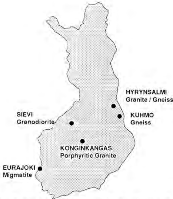
Fig. 3. The investigation areas for the selection of repository site for spent fuel.
