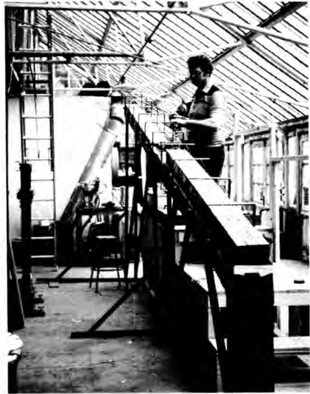
Fig. 16. Large Soil Beam Used for Final Selection of Diatomaceous Earth as Conductive Layer Material.
