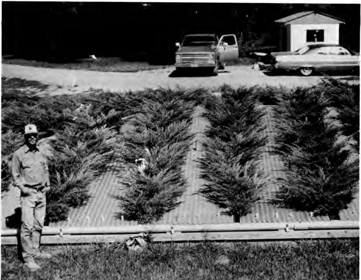
Fig. 5. Bioengineering Plots at Beltsville. Photo Taken in Fall of 1988, Two Years After Planting of Pfitzer Junipers. Run-off is 80% of Precipitation.
