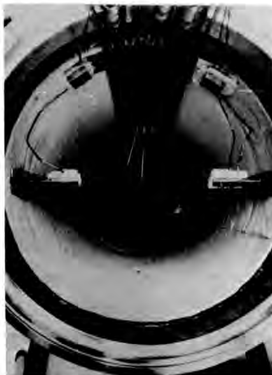
Fig. 1. View Into Canister #13 with Al 2 O 3 Insulation. Thermocouples are Guided by Means of Inconel Tubes. In the Vertical Position one can Observe the Arrangement of the Acoustic Emission Wave Guides.
