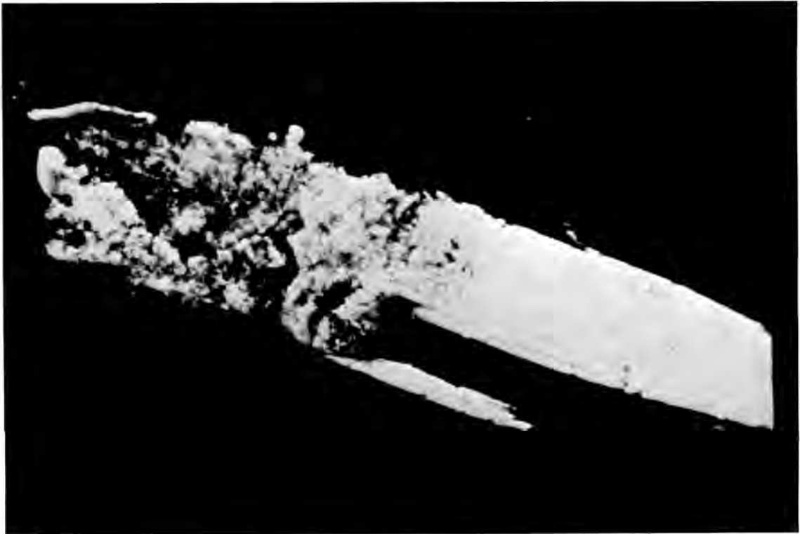
Fig. 2. Thermally Decomposed Polyhalite Crystal.
