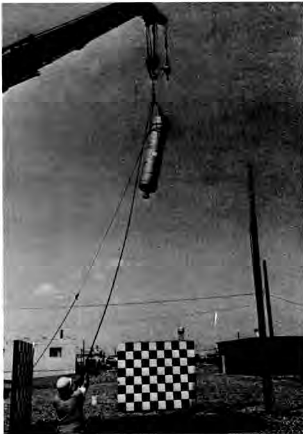
Fig. 3. Canister Elevated and Ready for Top Impact.
