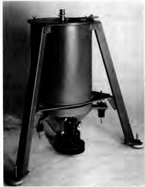
Fig. 2. Full-Scale Prototype Disposal Drum Centrifuge.
