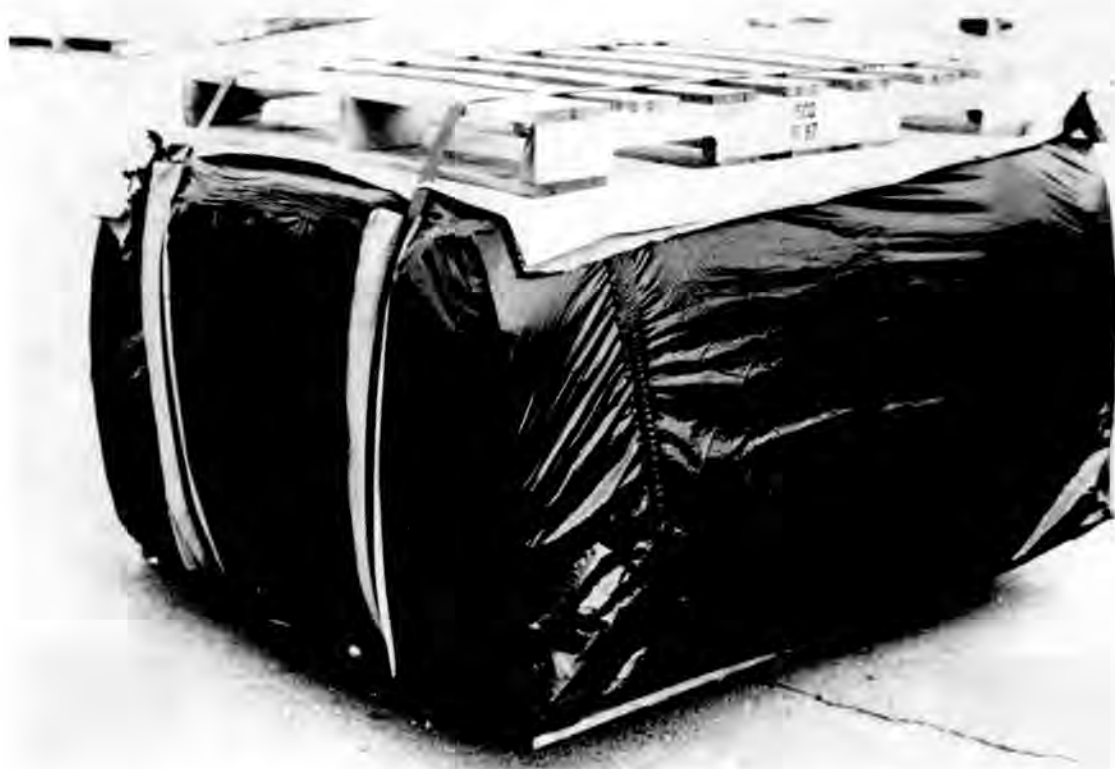
Fig. 3. Baled Trash Package Ready for Shipment to Disposal Site.
