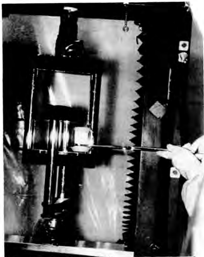
Fig. 2. Photograph of an EPICOR-II waste form being placed in the Instron compression testing machine.
