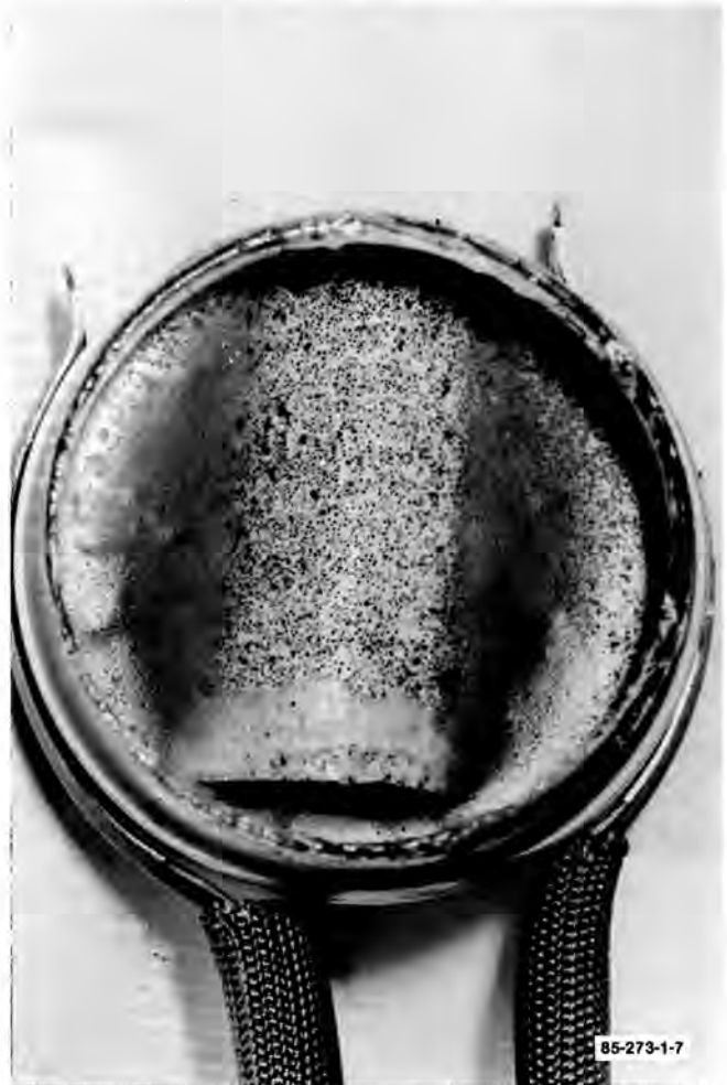
Fig. 5. Photograph of a VES waste form containing PF-7 wastes exposed to fungi in an agar-filled Petri dish during biodegradability testing.
