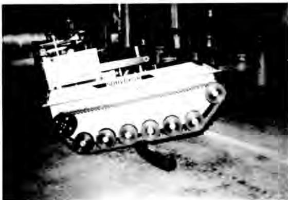
Fig. 2. Surveyor™ Surmounting the 4-inch Diameter Steel Pipe.
