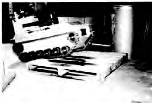
Fig. 3. Surveyor™ Starts to Surmount a 6-inch Height Wooden Pallet.
