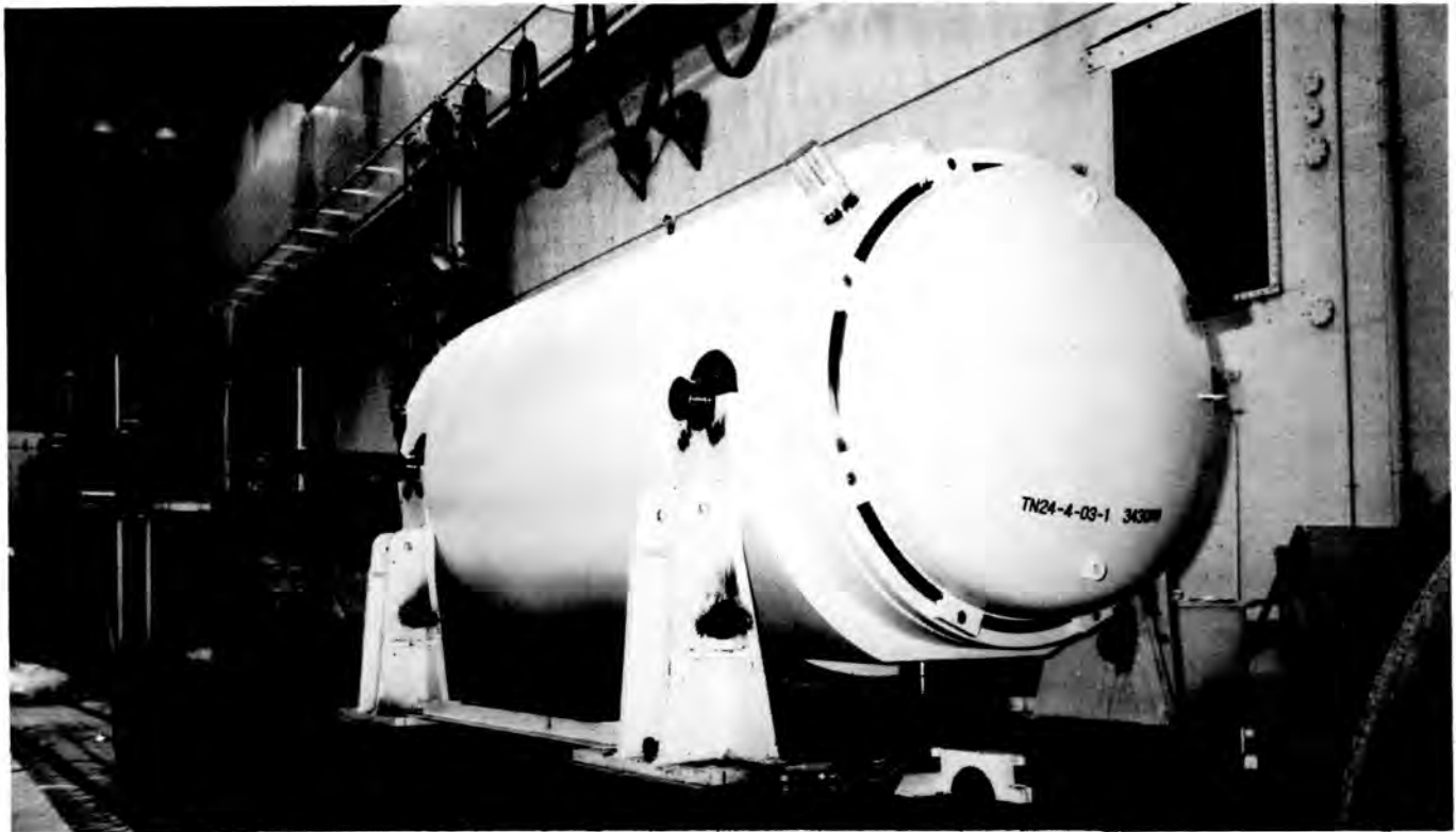
Fig. 3. Second Storage Cask (Transnuclear TN-24P).
