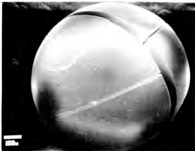
Fig. 4. SEM Photomicrograph of EPICOR-II Strong Acid Cation Resin Bead From PF-8#1 at 100 Magnification.
