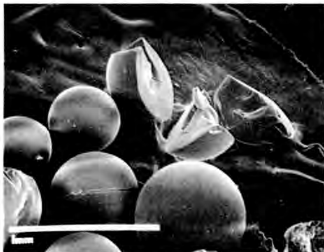
Fig. 6. SEM Photomicrograph of Other EPICOR-II Strong Acid Cation Resin Beads From PF-8#3 at 50 Magnification.
