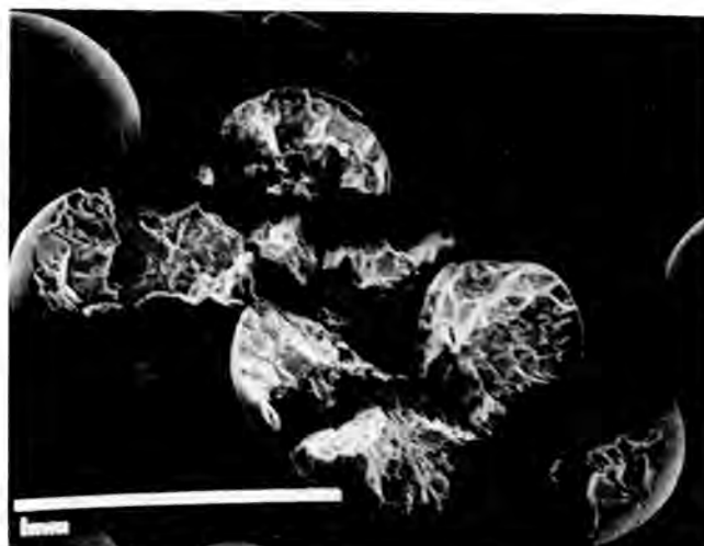
Fig. 5. SEM Photomicrograph of EPICOR-II Strong Acid Cation Resin Beads From PF-8#3 at 50 Magnification.
