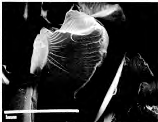
Fig. 7. SEM Photomicrograph of EPICOR-II Phenolic Cation Resin from PF-8#2, Showing a Closeup of One Resin Particle at 50 Magnification.
