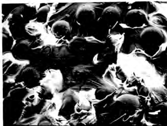
Fig. 3. Mixed bed resin to bitumen ratio = 50:50 w%. Stored dry in a refrigerator for ca 4 years. Water content 4.9%. SEM 35x. The pictures show the preferential orientation of the cracks from bead to bead. Also the diameter of the relatively dry beads can be measured fairly accurately.
