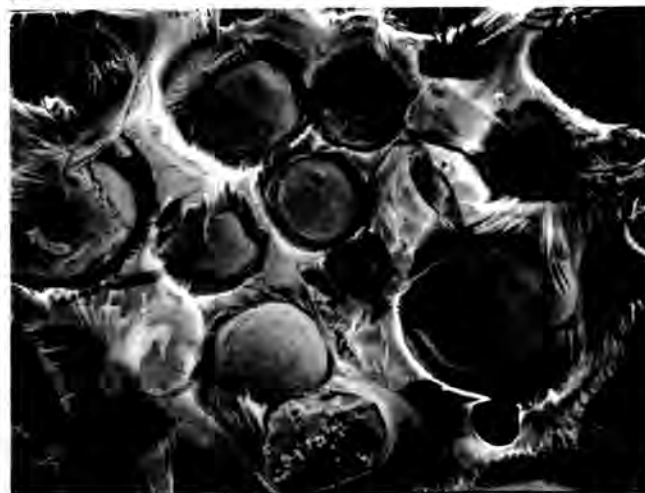
Fig. 4. A similar sample as in Fig. 3, but stored in contact with water. Water content 24.2%. Note the swelling of the beads and also the pores formed.
