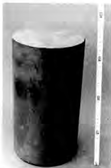
Fig. 5 Scale-up Solidified Product (180 mm diameter x 350 mm height)
