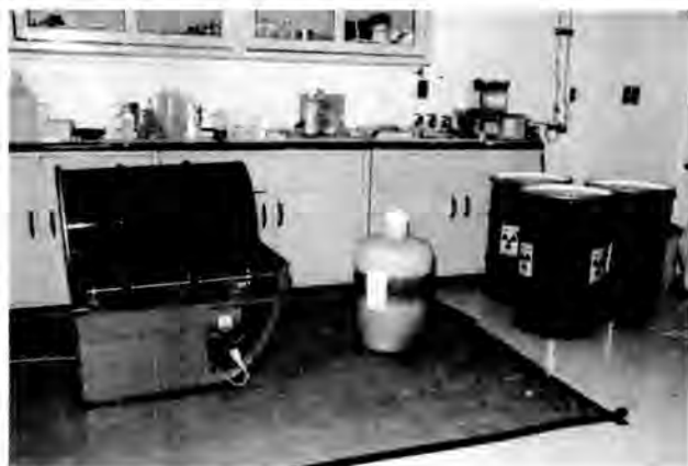
Fig. 4. Drum Roller Cementation Equipment.
