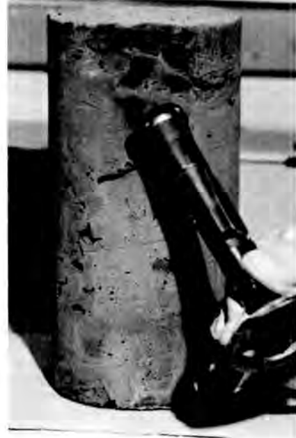
Fig. 16. Cement Solidified Solvent Product with 35% TBP-NPH Quits Burning as Soon as Burner is Removed.
