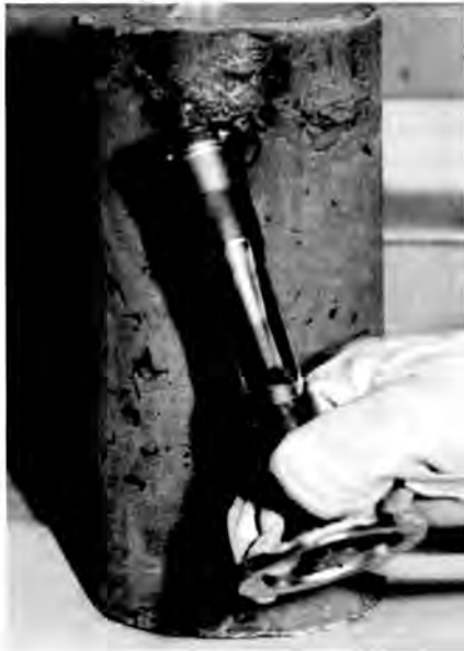
Fig. 15. Cement Solidified Solvent Product with 35% TBP-NPH Burns when Burner is Applied.
