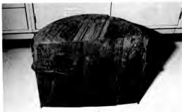
Fig. 12. A Quarter Section of Cement Immobilized Organic Liquid Waste.
