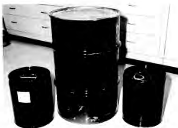
Fig. 14. Cement Solidified TBP-Dodecane Solvent Waste.
