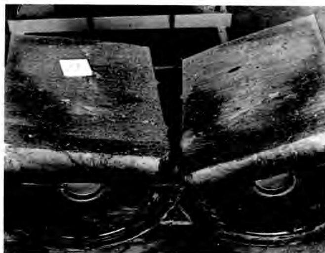
Fig. 3b. Solid Ash Drum with Sand Backfill
