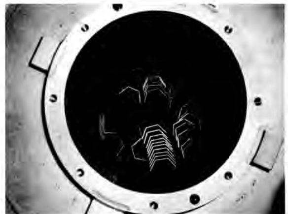
Fig. 4. Demonstration 19-Inch Diameter DSWC Single-Compartment Insert Packed with Slit Duct Sections
