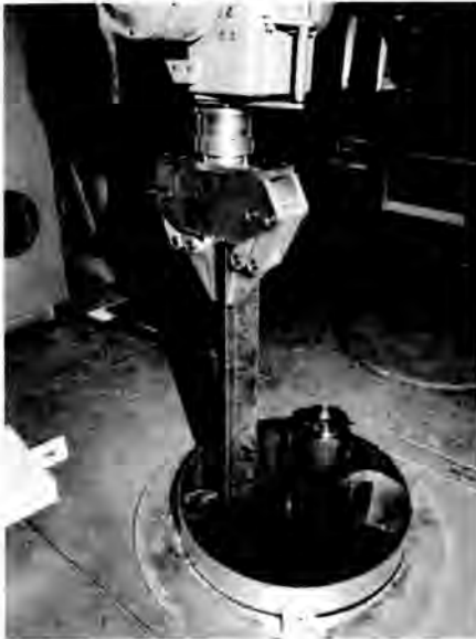
Fig. 5. Remote Loading of Waste Components by Electro-Mechanical Manipulator
