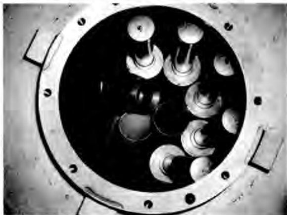
Fig. 7. Demonstration of Waste Packaging in DSWC Single Compartment Insert
