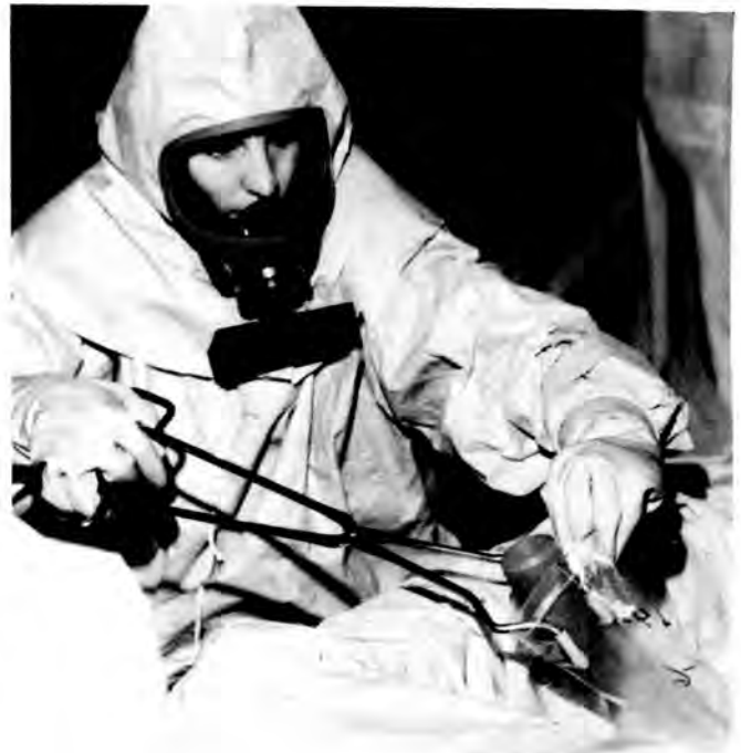
Fig. 4. Photograph showing an EPICOR-II waste form being placed in a plastic bag after the gamma irradiation portion of the irradiation stability testing. [Note the anti-contamination precautions taken by the technician.]
