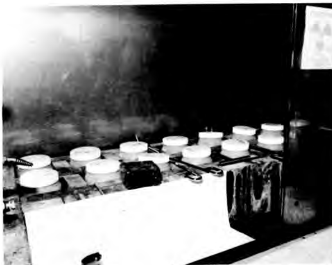
Fig. 3. Photograph of EPICOR-II waste forms in the leachate containers during leachability testing. [Note the lead brick shielding required to reduce radiation exposure to personnel.]
