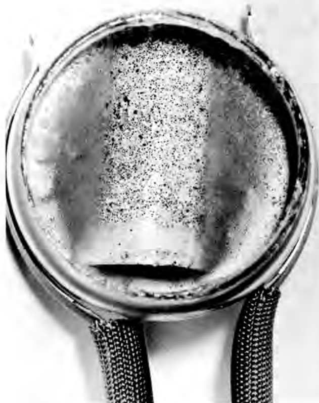
Fig. 5. Photograph of a VES waste form containing PF-7 wastes exposed to fungi in an agar-filled Petri dish during biodegradability testing.
