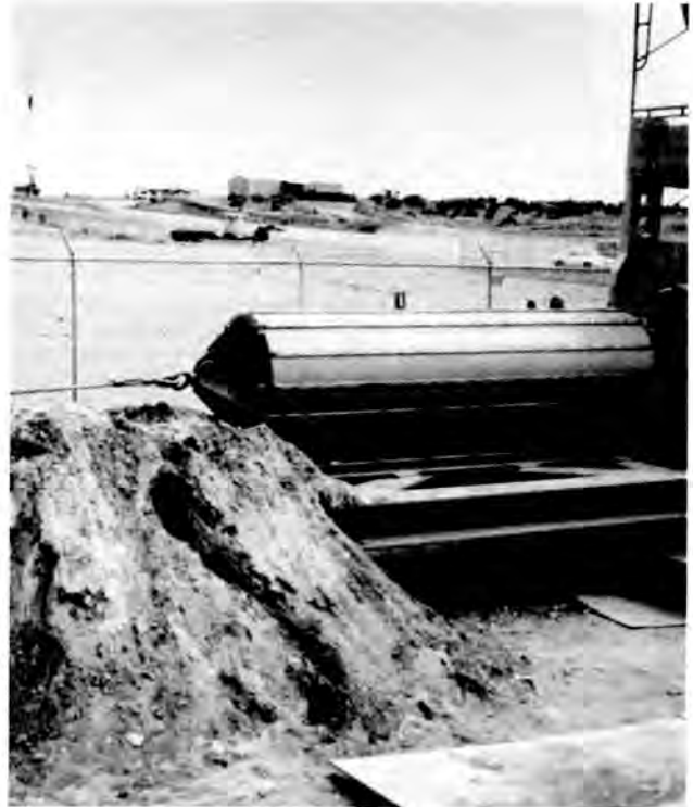
Fig. 7. Disposable liner removal during dry run demonstration of NTS handling equipment.
