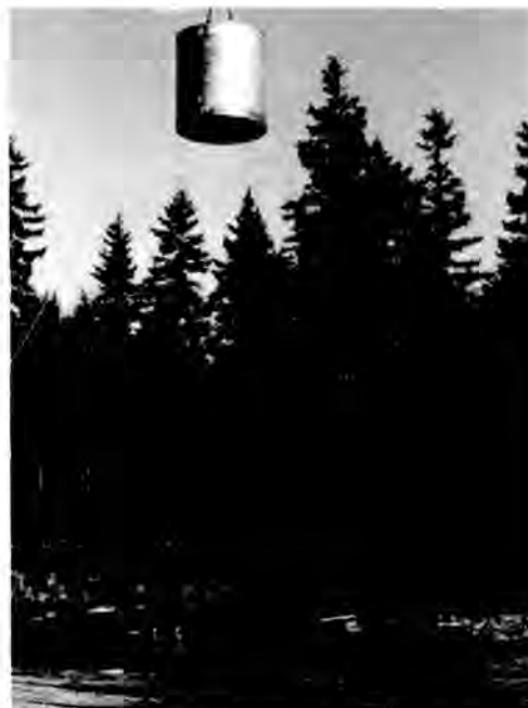
Fig. 2. Twenty-Five Foot Flat Bottom Drop.
