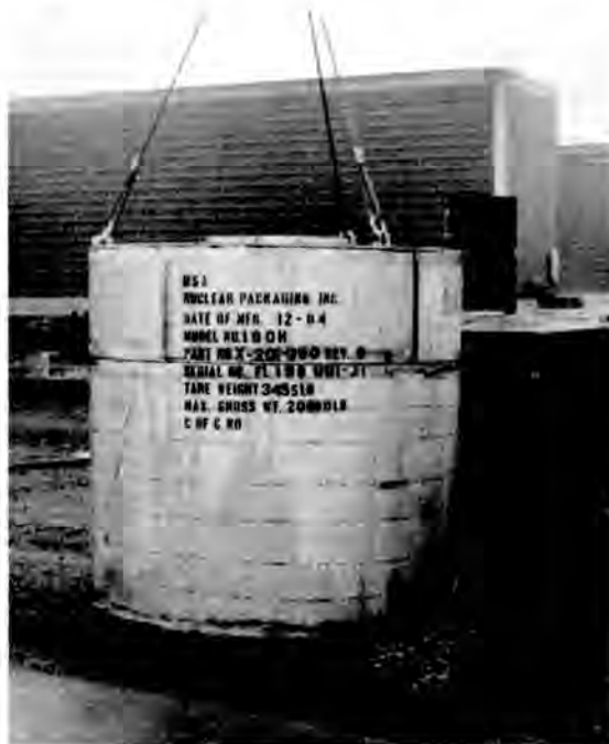
Fig. 1. Completed Enviroalloy Container.
