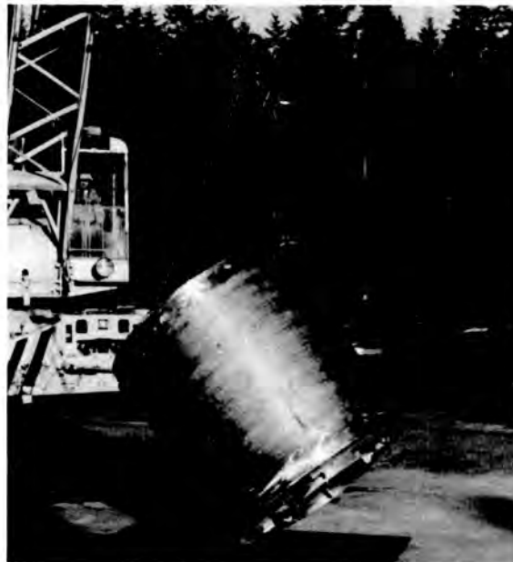
Fig. 4. Four Foot Top Corner Drop on Unyielding Surface.
