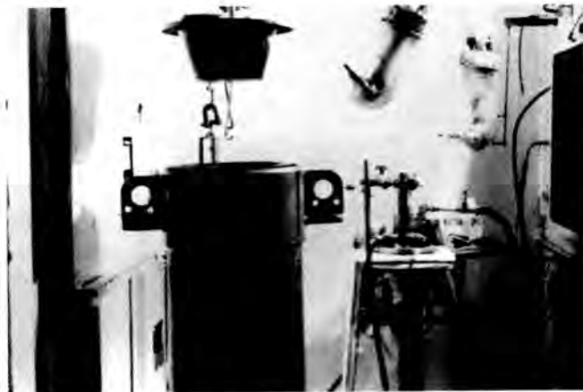
Fig. 4. Welding fixture and transport cask setup in cell prior to loading waste.
