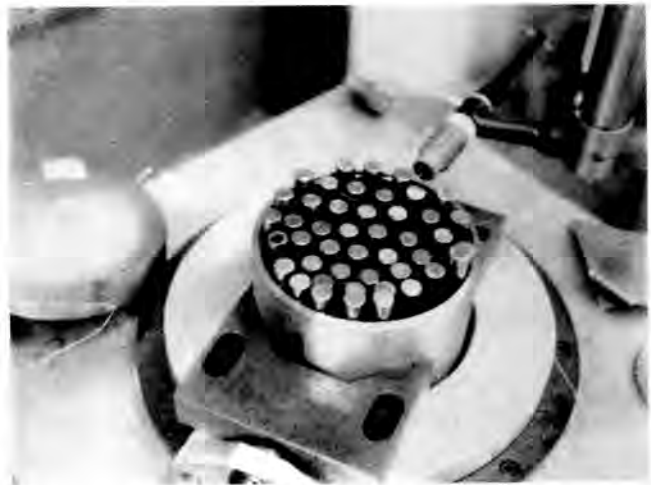
Fig. 6. Prototype container loaded with simulated waste.
