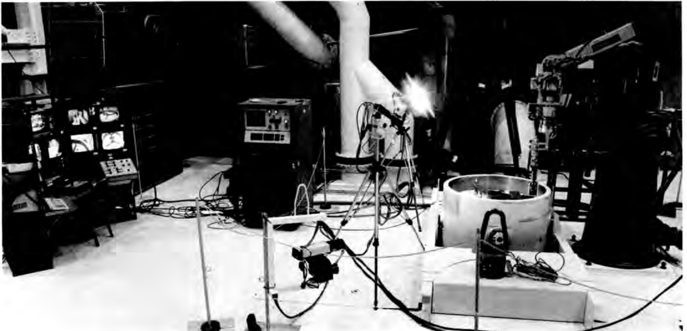
Fig. 1. Telerobotic Workstation with Cask Mockup in Support Fixture.
