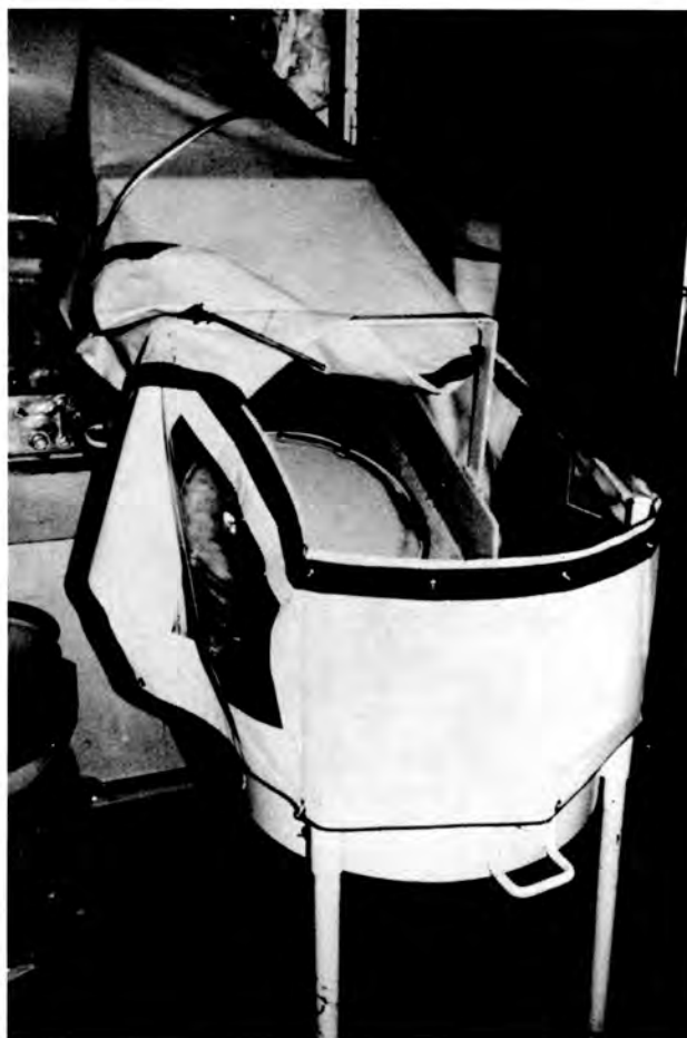
Fig. 6. Drum After Crushing.
