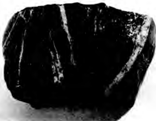
Fig. 5. Drill core sample of planar laminated siltstone from the Pumpkin Valley Shale illustrating abundant jointing. Note that joints are filled with secondary calcite.
