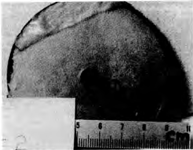
Fig. 11. Photograph of the interior surface of Section 2 from liner PF-16 showing a nearly defect-free coating.
