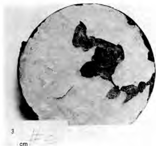
Fig. 7. Photograph of the interior surface of Section 3 from liner PF-3 showing coating blisters and areas where coating is missing.
