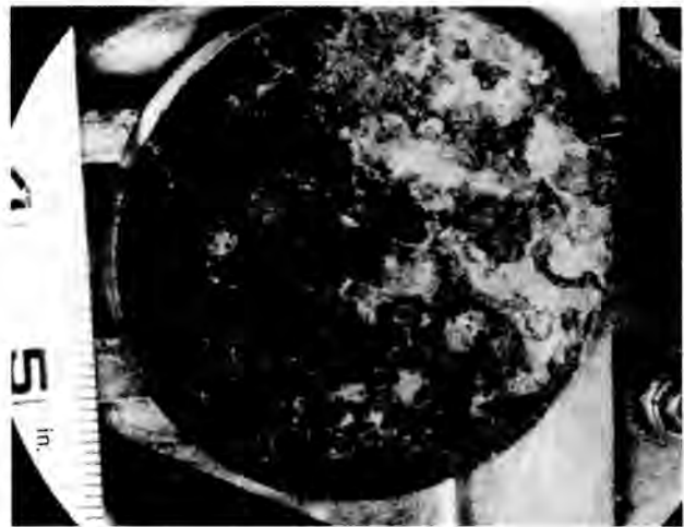
Fig. 5. Photograph of the interior surface of Section 1 from liner PF-3 showing a heavy deposit of corrosion products and residual resin.
