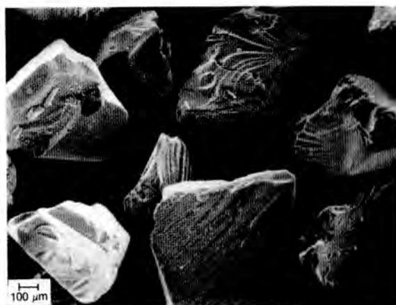
Fig. 7. SEM photomicrograph of Epicor unirradiated phenolic cation resin at 50 magnification.
