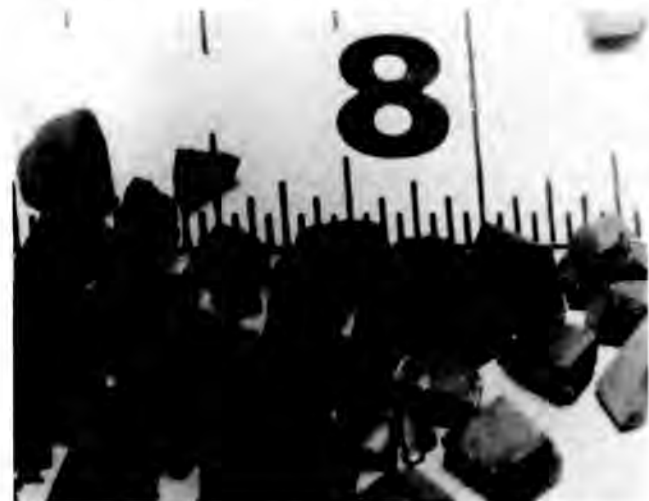
Fig. 4. Point Beach Spent Fuel After 965 h at 230^\circ C Prior to Formation of Fine Fragments.
