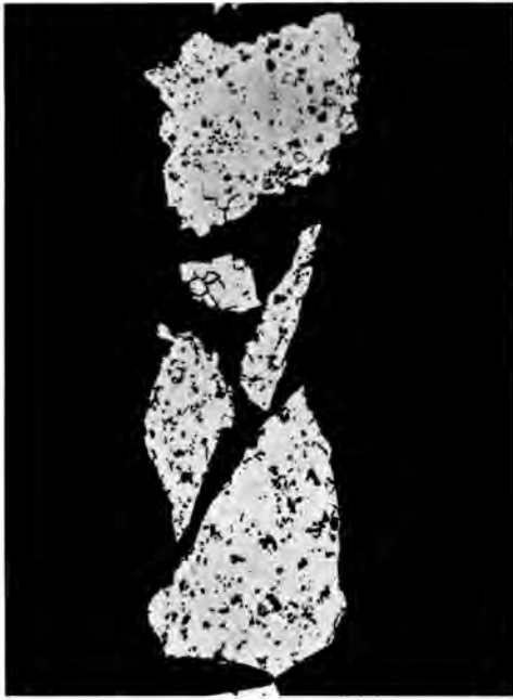
Fig. 5. As-polished cross-section of the pulverized fuel oxidized in +14.5°C dew point air at 225°C for 356 hours. Note the grain boundaries are usually seen only in etched UO 2 (250X).
